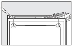
First screw the soft-close mechanism onto the appliance side, then onto the handle side ③, pushing it firmly towards the appliance.
